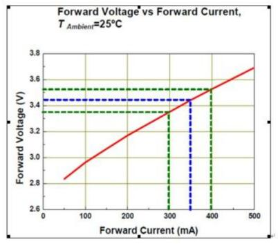
The output current  $I_o$  of LED power supply is350mA. Then according to the above diagram, the working voltage  $V_o$  of a single LED is 3.44V.
