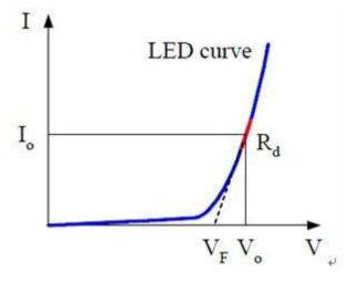
Io is working current, which should be set as the rated current of measured LED power supply.
