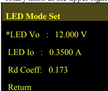
LED  $V_o$  : LED power supply working voltage
