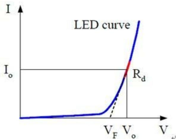
$I_o$  is working current, which should be set as the rated current of measured LED power supply.
